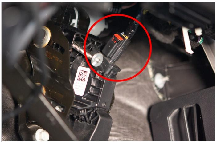
3. If the connector has a locking tab, slide the locking tab outwards to unlock. This will expose a black plastic button you will pinch to unlatch. Remove the connector from the accelerator pedal.
