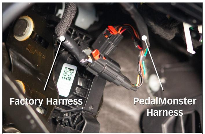
4. Connect the female PedalMonster plug to the accelerator pedal. Connect the male PedalMonster connector to the vehicle's female connector. Ensure both male and female connectors on the PedalMonster module are securely connected to the vehicle's connectors.
